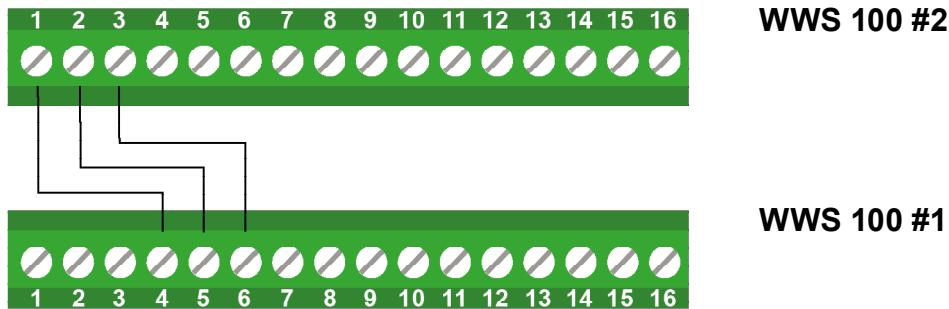
The WWS 100 Sensor is connected to the 5X or 6X on the panel (the input for break glass unit or Master-Slave connection).
