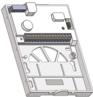
Open the box at the bottom and remove the front cover! Unplug the ribbon cable
