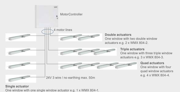
Up to four windows with each one window actuator can be connected e.g. 4 x WMX 804-1.
