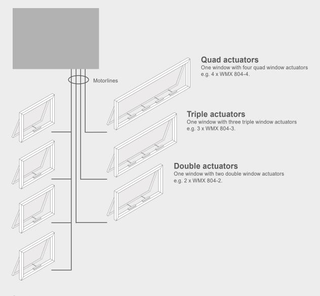
**Single actuator** One window with one single window actuator e.g. 1 x WMX 804-1. Up to four windows with each one window actuator e.g. 4 x WMX 804-1 can be connected.
